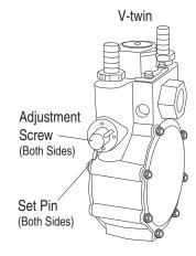
6. When the highest frequency is reached maximum power has been set. From this point, turn both adjustment screws 1/4 turn clockwise. The regulator is now set.
